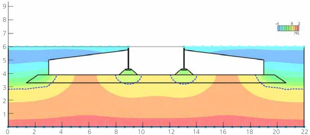
Figure 13. Ground temperature distribution simulated with the FEM software TEMP/W.
