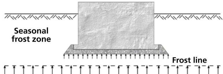
Figure 8. Normal forces acting on a shallow foundation (Andersland & Ladanyi, 1994).
