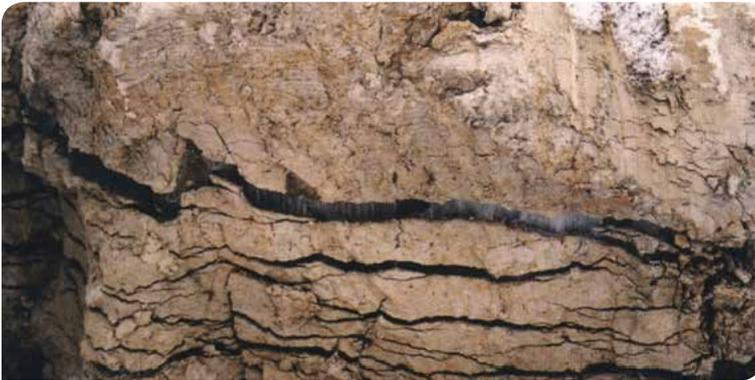
Figure 5. Ice lens in a silty soil.
