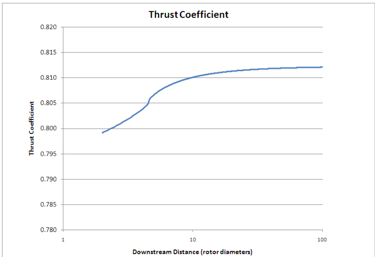
Figure 4 – Variation of Rotor Thrust Coefficient with Downstream Distance for the Crank-Nicolson method ( C_t = 0.8 , I = 10\% ).
