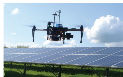
Thermographic imaging using a drone
